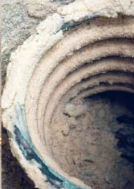
Hot water cylinder with hardwater scale
