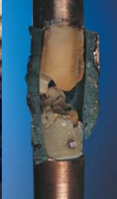
15mm copper pipe choked with hardwater scale
