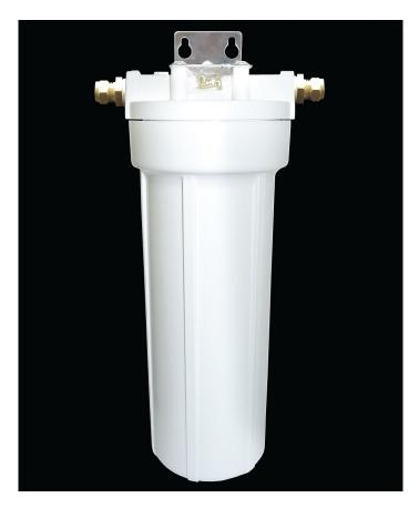
**IMPORTANT:** Maximum operating pressure rating is 95psi, we recommend the fitting of a pressure regulator if feed pressure is expected to exceed 90psi. Ambient temperature operating range is 5°C to 40°C. Protect system from cold, frost and excess heat.
